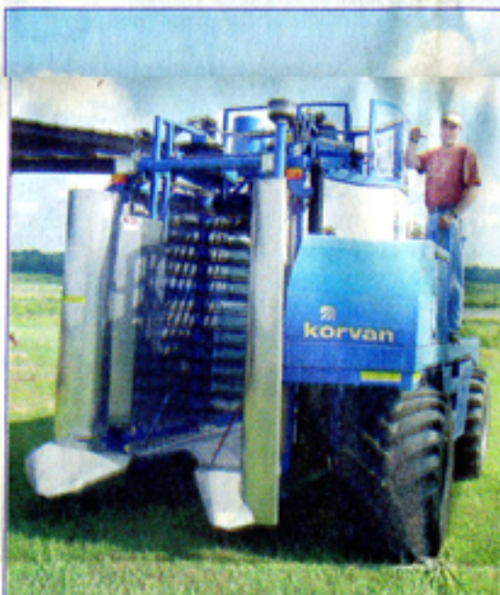
This new monster machine is now used to harvest blueberries from 55,000 bushes at Hillcrest Blueberry Farm. The bushes are mechanically shaken and doliied up a track that dumps them into lugs which are then carried to the processing room for further handling.
